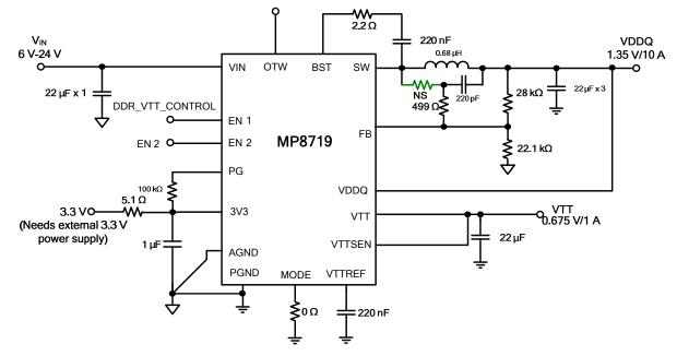
Figure 14: Typical DDR Application Circuit, VIN = 6V - 24V,  $V_{OUT} = 1.35V$ ,  $I_{OUT} = 10A$ , with VTT fs = 700kHz DDR Application Cover 5V VIN Application
