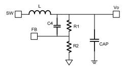
Figure 6: Simplified Output Circuit
